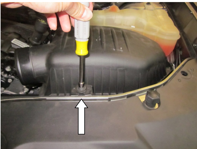
i) Loosen and remove the M6 bolt securing the air box. The M6 bolt will be reused in step 3j).
