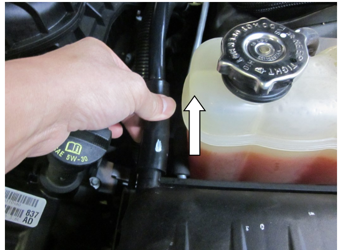
h) Detach the valve cover breather hose from the air box that will be reused in step 3n).
