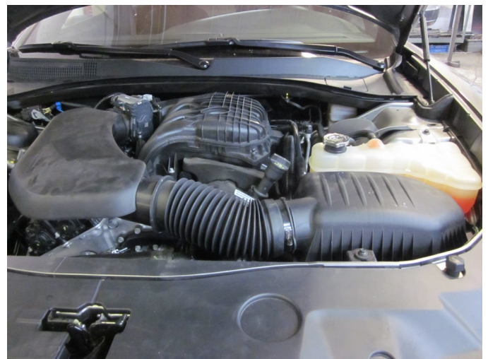
b) Remove the engine cover by pulling straight up.
