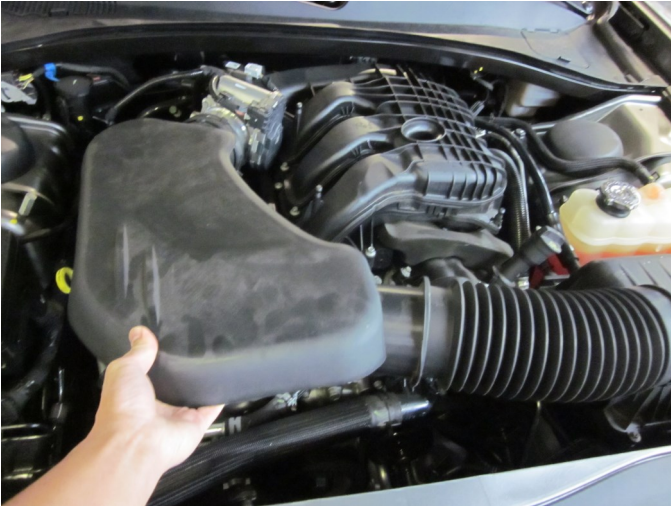
g) Detach and remove the factory air intake hose from the throttle body and air box.
