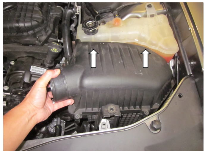
j) Pull the air box straight up to remove it from the engine bay.
